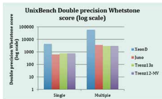
1: UnixBench, Whetstone test results for various devices under test (log scale)
